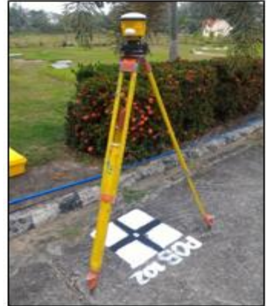
Figure 3.2 -1 Ground Control Survey using a survey grade GNSS
